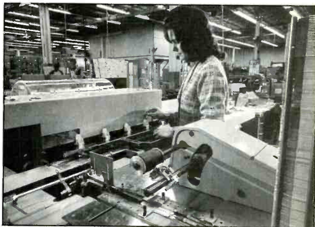
In this operation, ECG replacement semiconductors are packaged in boxes by equipment that imprints type numbers and basing diagrams of the devices on the individual cartons. The machine indexes 40 times per minute and can accommodate all semiconductor carton sizes.
