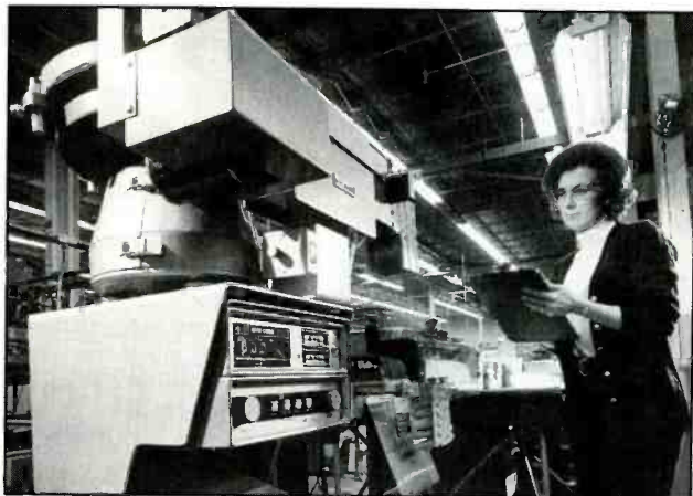
This Rapid Pack equipment automatically loads ECG replacement semiconductor products into individual plastic packages, imprints the type number on the label and seals the plastic bag for storage or shipping. Rapid Pack machines perform this operation 32 times per minute.
